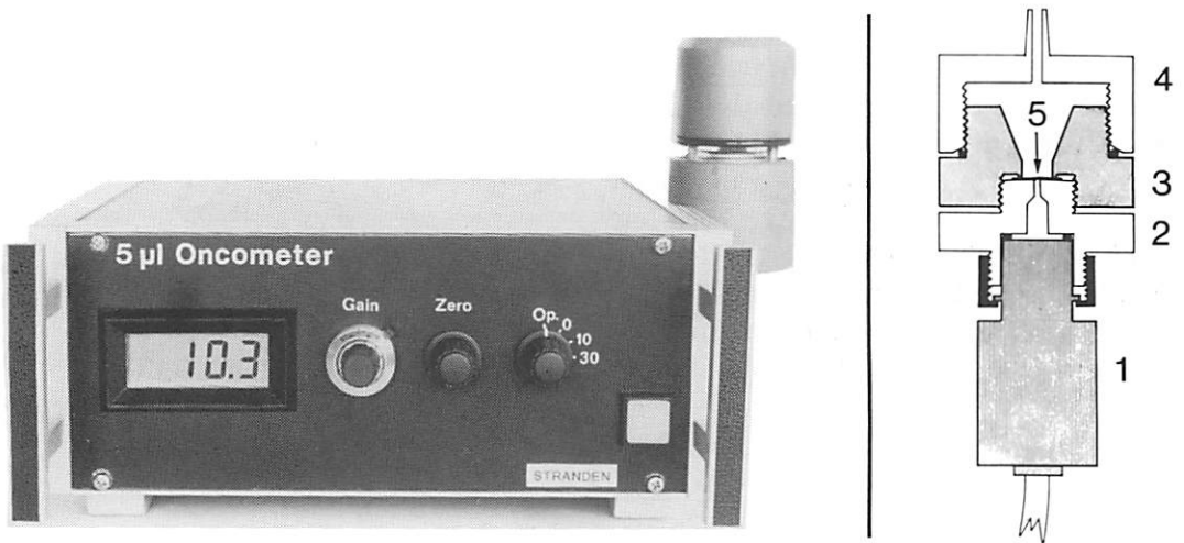
Fig. 3. «5 µl Oncometer» (1): Statham pressure transducer (P 23 Db) with low volume displacement ( 0.04 \text{ mm}^3/100 \text{ mm Hg} ), (2): reference chamber filled with isotonic saline solution, (3): sample chamber, (4): calibration connector, (5): dialyzing membrane with protein cutoff at MW 30000.
